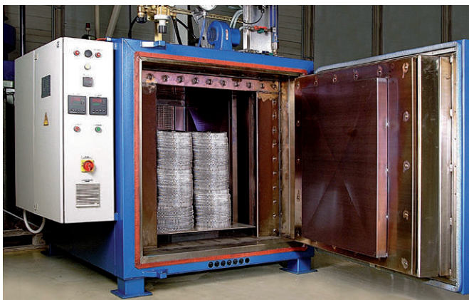
Anlassofen · Tempering Furnace
